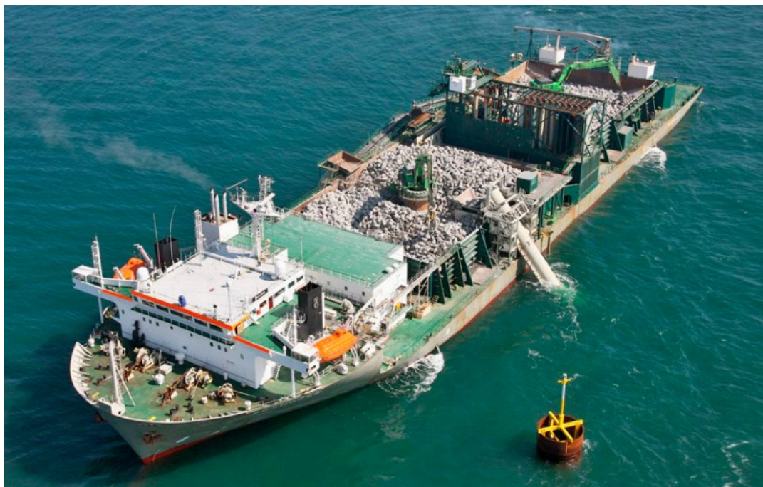
Figure 25 Typical rock placement vessel (source; Boskalis)
